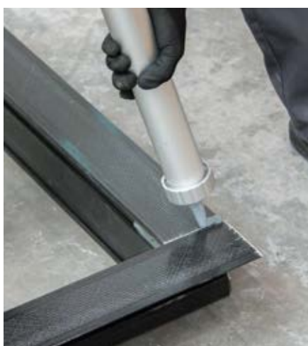
07 Apply the adhesive to all connection joints
